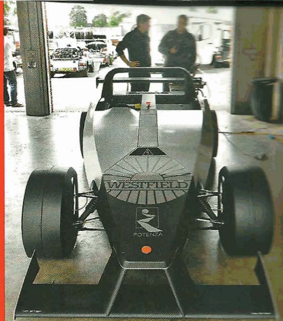
Plug and play: racer takes an hour to charge for 30-mile range
