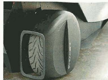
Aerodynamic wheel covers cut drag
